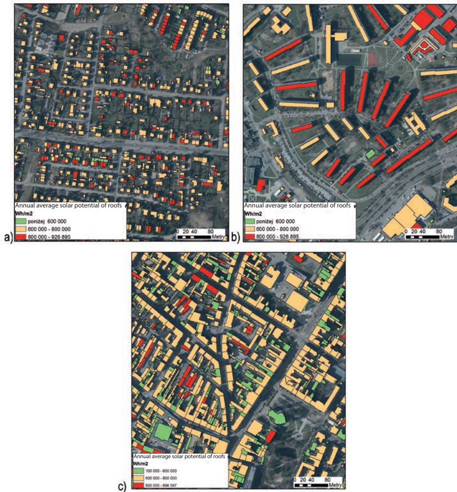
Fig. 7. The solar potential of the roofs of the buildings in Wh/m 2 in Bydgoszcz: a) in single-family houses settlement; b) in multi-family houses settlement; c) in the city centre
