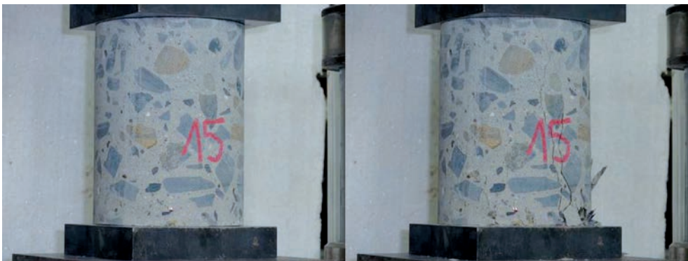
Figure 7 FRC specimen before test (left) and after test (right)
