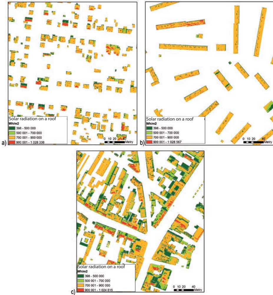
Fig. 6. The global radiation values for the roofs of the buildings on fragments of the analysed areas: a) single-family houses settlement, b) multi-family houses settlement, c) city centre.
