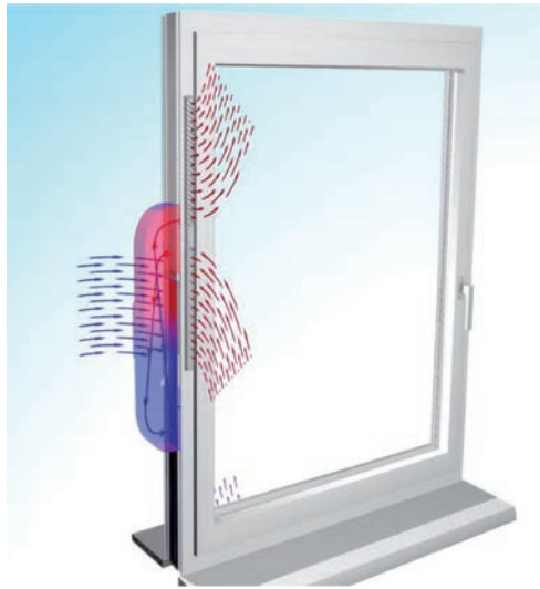
II. 3 Ventilation in the i-Tec Smart Window [12]
